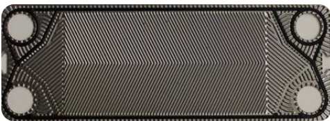
AFTER CLEANING with VARTECH ISC: Varnish film cleaned
